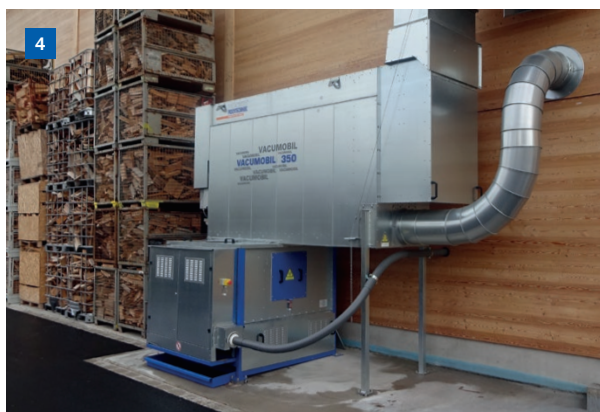
4 Vacumobil 350 with weatherproof enclosure for briquette press operation
