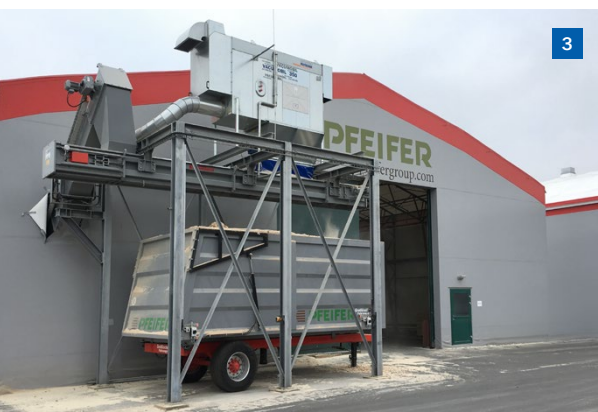
1 Vacumobil 350 with rotary airlock discharge into large waste containers
